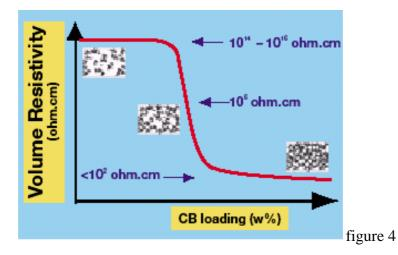
These additives are widely used for applications which demand an antistatic or semiconductive compound and can be used with almost all polymers. The use of carbon fibers allows to combine antistaticity with excellent mechanical characteristics and a good level of autolubrication.
